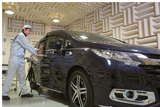
Testing using psychoacoustic technology to monitor the closing sound of car doors in an anechoic room (Mitsui Kinzoku ACT).
